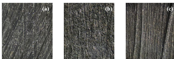
Figure 4 – Micrographs (×50) of the carbon steel surface after 24 hours of immersion in 1.0 mol·dm -3 HCl solution: before immersion (a), in the absence (b) and in the presence (c) of aqueous extract of R. nigrum leaves at a concentration of 1,0 g·dm -3
