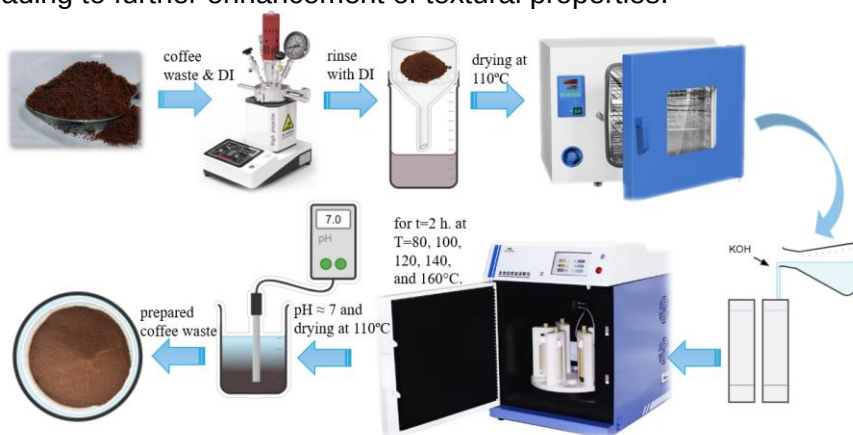
Figure 2 – Schematic illustration of carbon material synthesis from coffee waste
