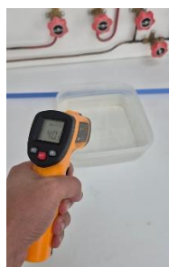
Figure 2 – Verification of water temperature before the experiment using an infrared thermometer
