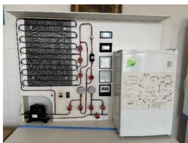
Figure 1 – General view of the «Kholodilnik-2» RTB 02.00.01 experimental stand
