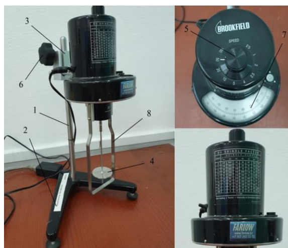
1 – bar; 2 – bed; 3 – clamp; 4 – rotor; 5 – speed regulator; 6 – screw; 7 – circle scale; 8 – protective frame
