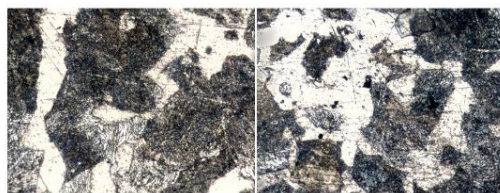
Figure 1 – Microstructure of 20GL steel before quenching
