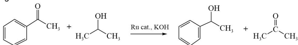
Figure 5 – Transfer hydrogenation of acetophenone
